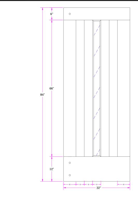
THIS DRAWING AND THE INFORMATION CONTAINED HEREIN IS PROPRIETARY TO TITLE 4975 2/8 x 7/0 SIMPSON DOOR COMPANY AND SHALL NOT BE REPRODUCED, COPIED OR DISCLOSED IN **Customer Layout** WHOLE OR PART, OR USED FOR MANUFACTURE OR FOR ANY OTHER PURPOSE WITHOUT THE WRITTEN PERMISSION OF SIMPSON DOOR COMPANY. D-4975-208-700-0700.dwg Revisions SCALE NTS PATTERN # 00000 LAYOUT 000 Rev. # Description Date by Whom DRAWN J. Decker DATE 2/23/2015
