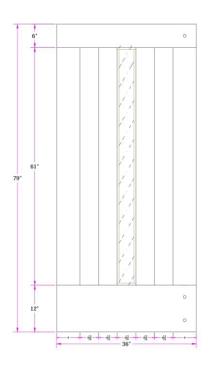
THIS DRAWING AND THE INFORMATION CONTAINED HEREIN IS PROPRIETARY TO TITLE 4975 3/0 x 6/7 SIMPSON DOOR COMPANY AND SHALL NOT BE REPRODUCED, COPIED OR DISCLOSED IN **Customer Layout** WHOLE OR PART, OR USED FOR MANUFACTURE OR FOR ANY OTHER PURPOSE WITHOUT THE WRITTEN PERMISSION OF SIMPSON DOOR COMPANY. D-4975-300-607-0700.dwg Revisions SCALE NTS PATTERN # 00000 LAYOUT 000 Rev. # Description Date by Whom DRAWN J. Decker DATE 07/28/2015
