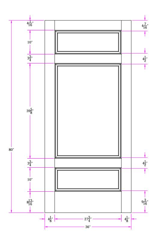
THIS DRAWING AND THE INFORMATION CONTAINED HEREIN IS PROPRIETARY TO 85 3/0 x 6/8 SIMPSON DOOR COMPANY AND SHALL NOT BE REPRODUCED, COPIED OR DISCLOSED IN **Customer Layout** WHOLE OR PART, OR USED FOR MANUFACTURE OR FOR ANY OTHER PURPOSE WITHOUT THE WRITTEN PERMISSION OF SIMPSON DOOR COMPANY. DRAWING NO. D-85-300-608-0300 Revisions LAYOUT PATTERN # 11612 NTS Rev. # by Whom DATE 08/05/2011 S. Beerbower **Simpson®**
