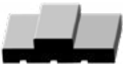
Standard Flat Jamb with Applied Stop
