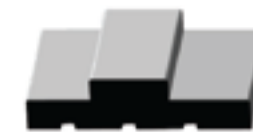
Standard Flat Jamb with Applied Stop
