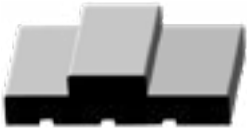
Standard Flat Jamb with Applied Stop
