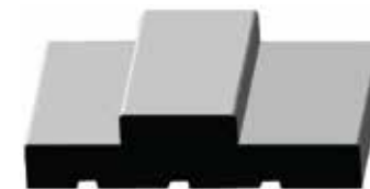
Standard Flat Jamb with Applied Stop
