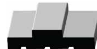
Standard Flat Jamb with Applied Stop
