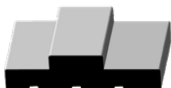
Standard Flat Jamb with Applied Stop
